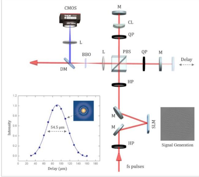
Figure 2. Schematic diagram of the implemented experimental setup, where the key components are the mirror (M), lens (L), cylindrical lens (CL), polarizing beam splitter (PBS), half-wave plate (HP), quarter-wave plate (QP), spatial light modulator (SLM), dichroic mirror (DM), and camera (CMOS).
