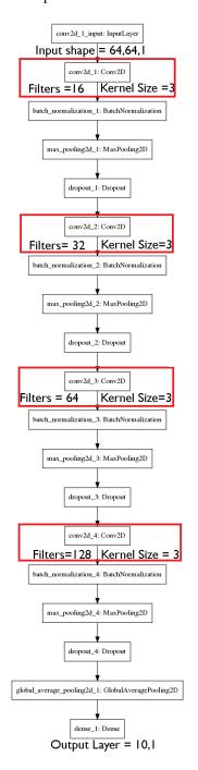
Figure 5. The CNN architecture used for digit recognition.
