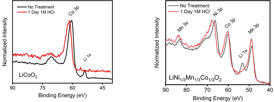
Fig. 3: (Left) XPS results for as-received  $\text{LiCoO}_2$  (LCO) and 1M HCl treated LCO showing the removal of Li and the shift in Co-3p peak. (Right) XPS results for as-received  $\text{Li}(\text{Ni},\text{Mn},\text{Co})\text{O}_2$  (NMC) and 1M HCl treated NMC showing the removal of Li and the shift in Ni-3p peak. Co and Mn peaks do not change with treatment.
