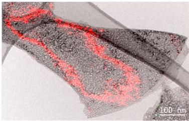
Fig. 2: Superposition of bright (grey) and dark field image (red) of a strong 220 diffraction peak characteristic of the rocksalt domains of a  $\text{LiCoO}_2$  nanoflake after annealing to  $350^\circ\text{C}$  showing that rocksalt domains occur primarily at the rim of the flake.
