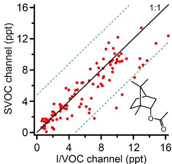
**Figure 6** Bornyl acetate measured on the I/VOC and SVOC channels of cTAG during FIREX-AQ. Dashed lines represent  $\pm 4.8$  ppt (3 times the I/VOC channel limit of detection for bornyl acetate). 96 % of data points fall within the region bounded by the dashed lines.  $R^2$  is 0.79.
