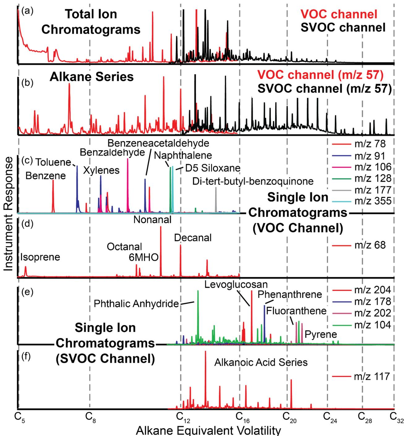
**Figure 7** Example chromatograms from cTAG. Panels (a) and (b) demonstrate the range of volatility covered by the two channels, including their overlap region. Single ion chromatograms (panels (c) through (f)) show examples of the compound classes observable by cTAG, including aromatics, polycyclic aromatic hydrocarbons, organic acids and anhydrosugars.
