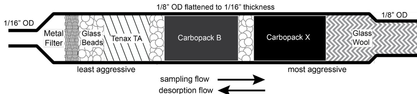
**Figure 2** Schematic of I/VOC collector. Semivolatile and lower volatility species, including particles, are captured on the metal filter. IVOCs are captured on the glass beads and Tenax TA, while the most volatile analytes including isoprene are retained by the more aggressive adsorbents. Flow is reversed for desorption so that the less volatile compounds never interact with the more aggressive adsorbents.
