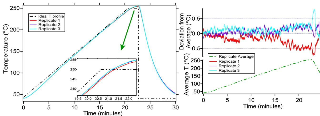
**Figure A2** Demonstration of reproducibility of temperature ramps on the miniature gas chromatographs. This leads to consistent elution times of compounds of interest, streamlining batch peak integration.
