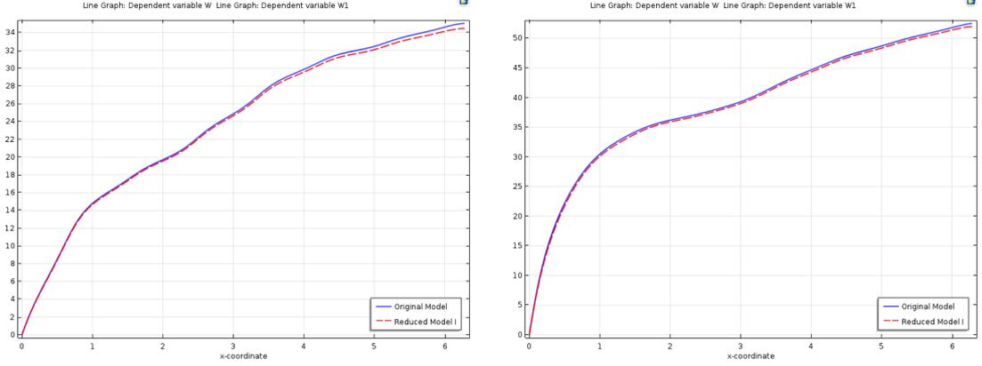
Figure 10: Coupled domain 1: comparison between the pressure distributions in the coupled fracture porous media domain, obtained using the original model and the Reduced Model I, for  $H = 0.01$ ,  $\beta = 0$  (left) and  $\beta = 100$  (right), respectively.
