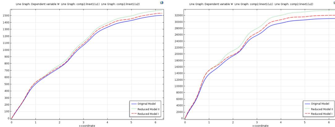
Figure 8: Fracture geometry 4: comparison between the pressure distributions inside the fracture, obtained using the original model, the Reduced Model I and the Reduced Model II, for  $\beta = 0$  (left) and  $\beta = 0.1$  (right), respectively.
