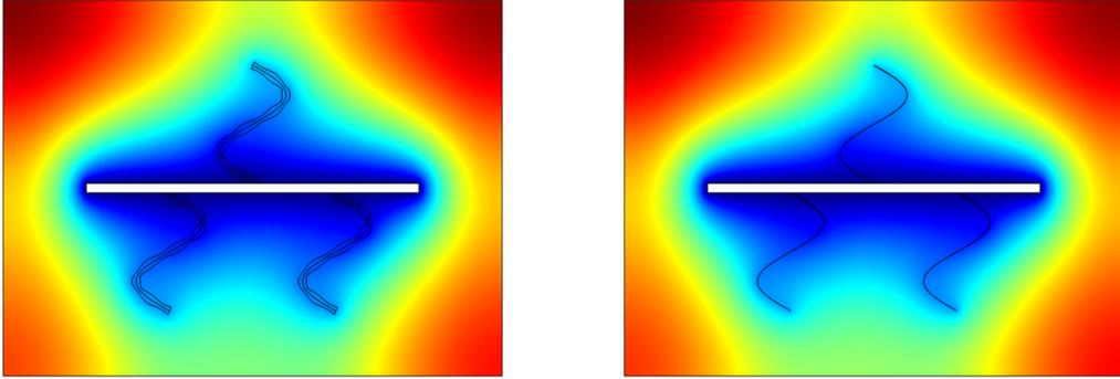
Figure 11: Coupled domain 2: pressure distributions in the coupled fracture porous media domain with  $H = 0.1$  and  $\beta = 1$ , obtained using the original model (left) and the Reduced Model I (right), respectively.
