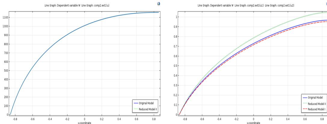
Figure 6: Fracture geometry 1: comparison between the pressure distributions obtained from the original model, the Reduced I and Reduced Model II for  $\beta = 0.1$ ,  $2h(u) = 0.025$  (left) and  $2h(u) = 1$  (right) respectively.
