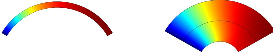
Figure 5: Fracture geometry 1: pressure distribution inside a thin fracture- $2h(u) = 0.025$  (left) and a thick fracture- $2h(u) = 1$  (right), obtained using the original model.
