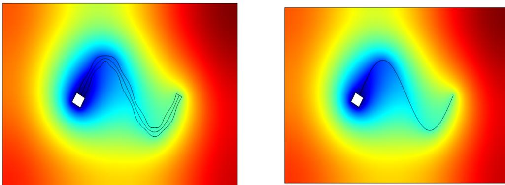
Figure 9: Coupled domain 1: pressure distributions in the coupled fracture porous media domain with  $H = 0.1$  and  $\beta = 0.001$ , obtained using the original model (left) and the Reduced Model I (right), respectively.
