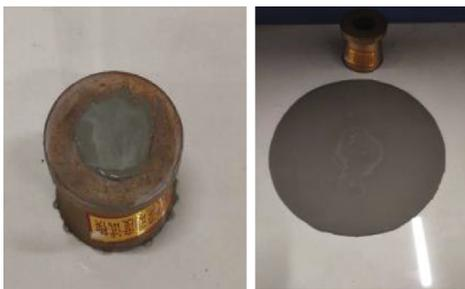
FIGURE 3: Cement fluidity test.
