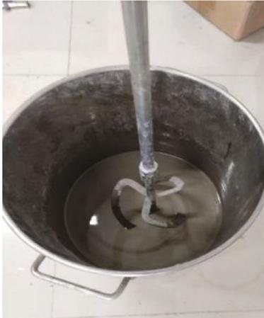
FIGURE 1: Borehole sealing material after mixing.
