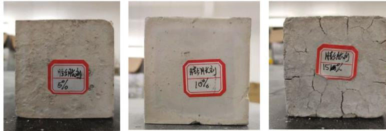
FIGURE 18: Effect of different dilatant dosages on test block.
