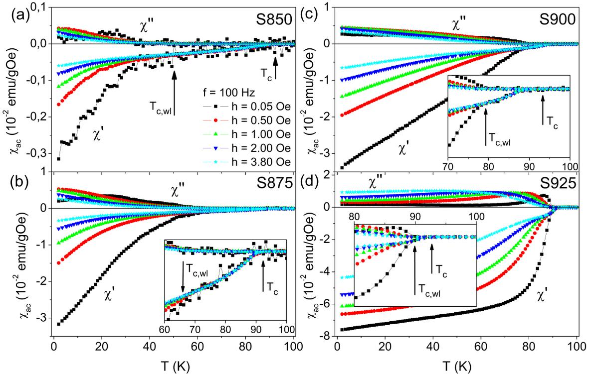
**Figure 5.**  $\chi_{ac}(T)$  measurements for  $h = 0.05, 0.5, 1, 2,$  and  $3.8$  Oe at  $100$  Hz and remnant dc field for the samples (a) S850, (b) S875, (c) S900, and (d) S925.
