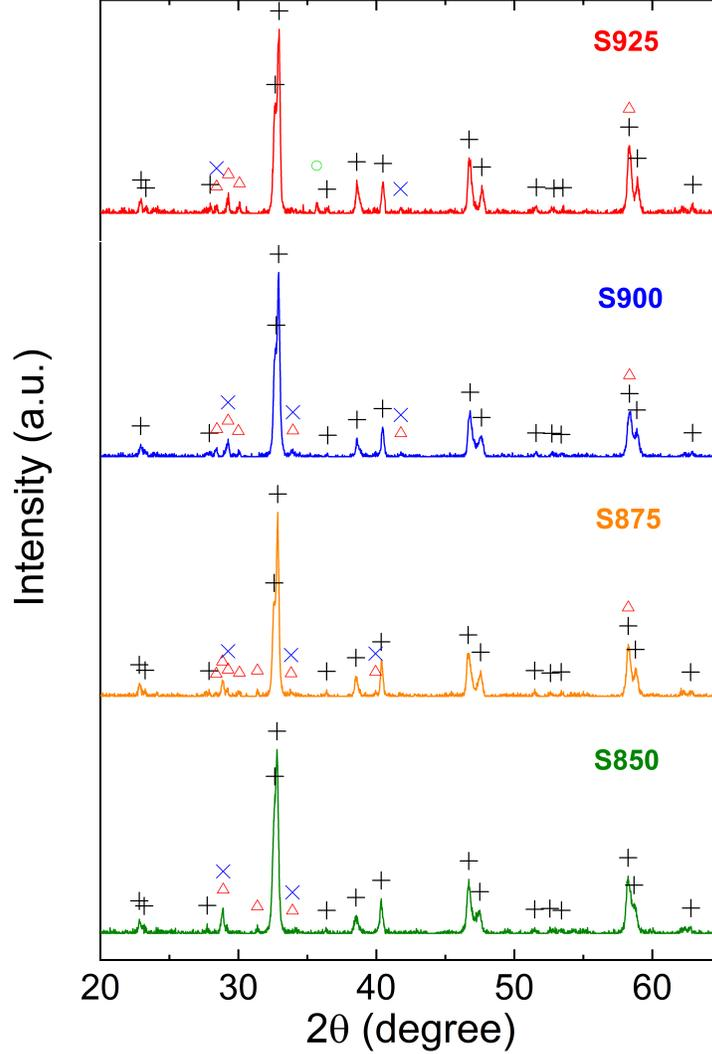
**Figure 4.** XRD analysis. Phase identification for all samples. Symbols represent the following phases: Y123 (+),  $\text{BaCuO}_x$  ( $\Delta$ ),  $\text{Y}_2\text{O}_3$  ( $\times$ ), and  $\text{CuO}$  ( $\circ$ ).
