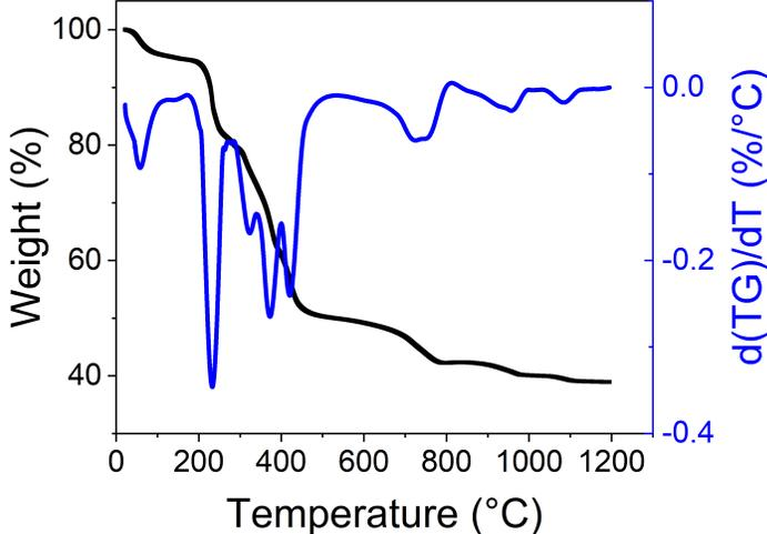
**Figure 2.** Thermogravimetric analysis (TG and DTG curves) of the polymeric precursor sample. Up to 500 °C, the weight loss and the DTG dips are related to water, solvent evaporation, and polymer elimination. Dips above 800 °C are related to crystallization of Y123 compounds.
