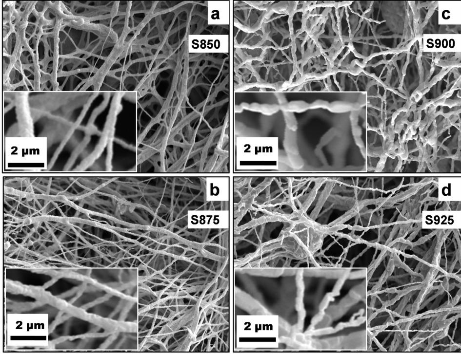
**Figure 3.** SEM images of Y123 samples subjected to different maximum sintering temperatures (a) 850 °C, (b) 875 °C, (c) 900 °C and (d) 925 °C.
