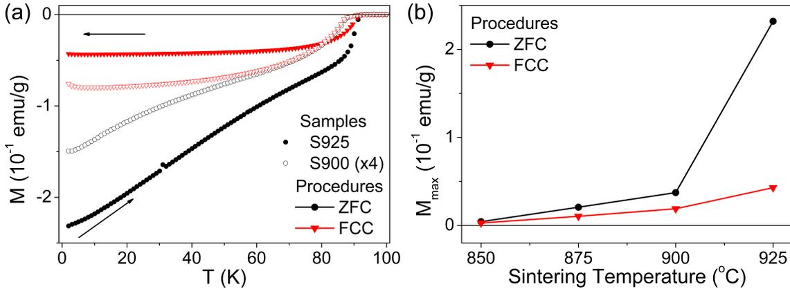
**Figure 6.** Dc magnetization response. (a) Temperature-dependent magnetization curves for the samples S900 ( $\times 4$  for better visualization) and S925 taken following ZFC and FCC procedures. (b) Absolute value of the dc magnetization at  $T = 2$  K obtained from ZFC and FCC curves as a function of the sintering temperature. In these cases, magnetization is given by the ratio of the magnetic moment to the sample mass.
