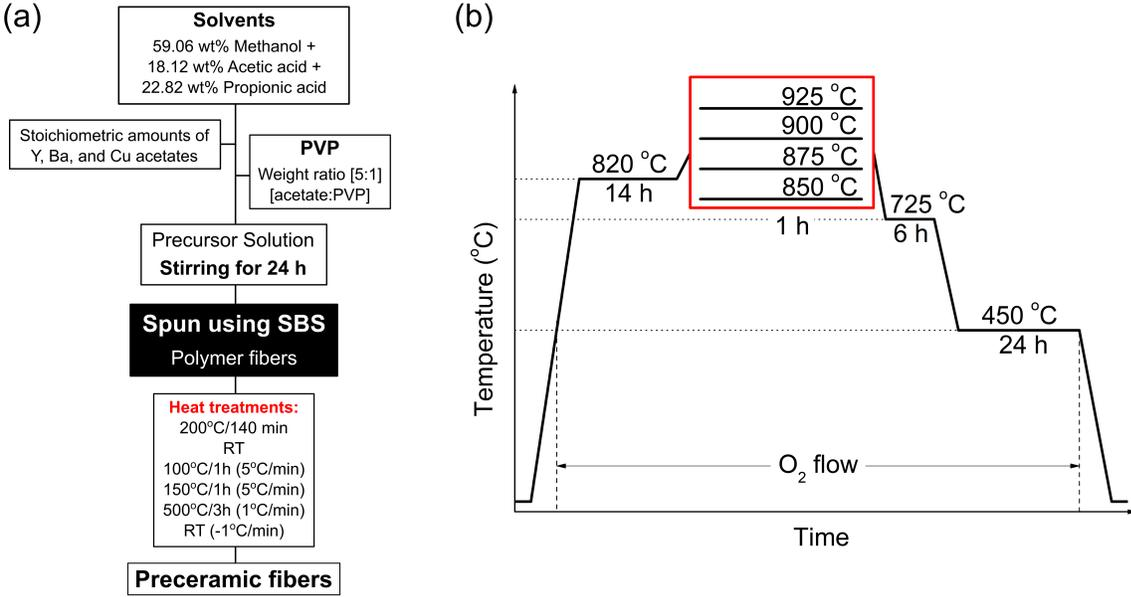
**Figure 1.** Sample preparation details. (a) Flowchart of the preceramic wire preparation. (b) Heat treatment for the samples S850, S875, S900, and S925.
