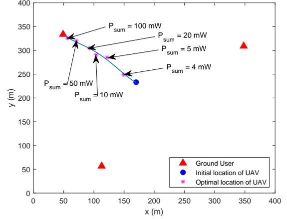
Fig. 1. The optimal UAV location with different values of  $P_{sum}$ .  $\eta = (1, 1, 1)$  bit/s/Hz.
