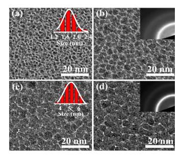
FIG. 1. Bright-field TEM images for  $\text{Ta}_x(\text{SiO}_2)_{1-x}$  films with x values of (a) 0.45, (b) 0.66, (c) 0.75, and (d) 0.8. The insets in (a) and (c) are the grain-size distribution histograms for the  $x \simeq 0.45$  and 0.75 films, respectively, and in (b) and (d) are the selected-area electron-diffraction patterns of the corresponding films.
