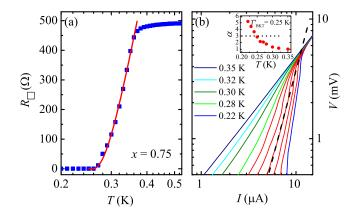
FIG. 3. (a) The sheet resistance  $R_{\Box}$  versus temperature T for the  $x \simeq 0.75$  film. The solid curve is the least-squares fits to the Halperin-Nelson formula. (b) Voltage versus current (in double logarithmic scales) measured at constant temperature ranging from 0.22 to 0.35 K for zero magnetic field, the steps are 0.01 K from 0.22 to 0.28 K. Inset:  $\alpha$  as a function of T. The dashed line represents the  $\alpha = 3$  line.
