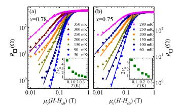
FIG. 6. Sheet resistance as a function of H- $H_{c0}$  in double logarithmic scales at different temperatures for (a)  $x \simeq 0.78$ , and (b)  $x \simeq 0.75$  films. The solid lines are least-squares fits to Eq. (2). Inset: The exponent  $2\nu_0$  in Eq. (2) as a function of T for the corresponding films.
