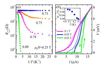
FIG. 5. (a) Logarithm of the sheet resistance as a function of  $T^{-1}$  from 1 down to 0.04 K at a field of 0.25 T for the  $x\simeq 0.73$ , 0.75, 0.78 and 0.80 films. (b) *I-V* curves for the  $x\simeq 0.75$  film measured at different fields. Inset:  $H_{c0}$  as a function of temperature for the  $x\simeq 0.75$  film.
