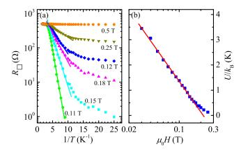
FIG. 4. (a) Logarithm of resistivity as a function of  $T^{-1}$  at different magnetic field for the  $x \simeq 0.75$  films. The symbols are the experimental data and the straight solid lines are least-squares fits to  $R_{\Box} = R_0(H) \exp(-U(H)/k_B T)$ . (b) Activation energy  $U(H)/k_B$ , obtained from the slopes of the solid lines in Fig. 4(a), as a function magnetic field for the  $x \simeq 0.75$  film. The solid line is the least-squares fit to Eq. (1).
