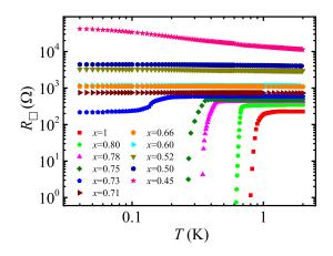
FIG. 2. Sheet resistance as a function of temperature from 2 down to 0.04 K for the  $\text{Ta}_x(\text{SiO}_2)_{1-x}$  films  $(0.45 \leq x \leq 1)$ .
