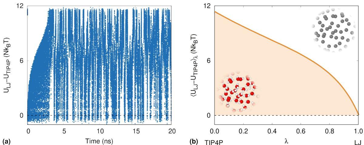
FIG. 4. Calculation of the free energy of liquid TIP4P water using a single-simulation thermodynamic integration. (a) Evolution of the collective variable  $\Delta U$  as a function of simulation time. (b) Integrand for the thermodynamic integration obtained through reweighting.
