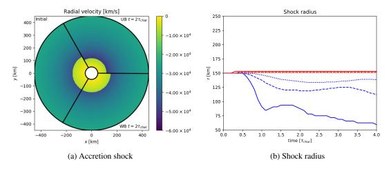
Figure 14: The left panel shows the radial velocity contour for resolution  $(N_r, N_\varphi) = (256, 512)$ . The right panel shows the shock radius as a function of time for un-/well-balanced (blue/red lines) for resolutions  $(N_r, N_\varphi) = (128, 256), (256, 512), (512, 1024)$  (solid, dashed, dotted lines).
