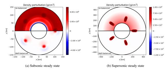
Figure 13: Small amplitude density perturbations on the subsonic (left panel) and supersonic (right panel) steady state. In both panels, the lower/upper plane show the results obtained with the un-/well-balanced schemes at resolution  $(N_r, N_\varphi) = (128, 256)$ , respectively. The color axis is clipped to highlight the absence of spurious deviations away from the perturbations for the well-balanced scheme.
