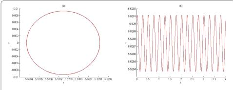
**Figure 1** The first picture shows the system response in the (x,y). The second shows the system response in the (t,x) over the time interval of  $0 \le t \le 50$ . The initial conditions are  $x_0 = 5.52907$ ,  $y_0 = 0$ ,  $t_0 = 0$
