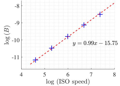
Fig. 3: log-log plot of the estimated first order coefficient  $B$  against the ISO speeds of the images used to estimate  $B$ . A straight line is fitted with a slope of 0.99
