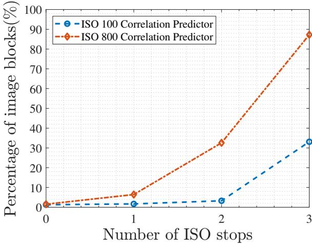
Fig. 6: A plot of the percentages of image blocks with  $d_1 - d_2$  smaller than 0 against the number of ISO stops the test image’s ISO speed is above the ISO speed of the images used to train the correlation predictor for a Canon M6. The percentage indicates the portion of the authentic image blocks at risk of being misidentified as tampered blocks by forgery detection algorithms.
