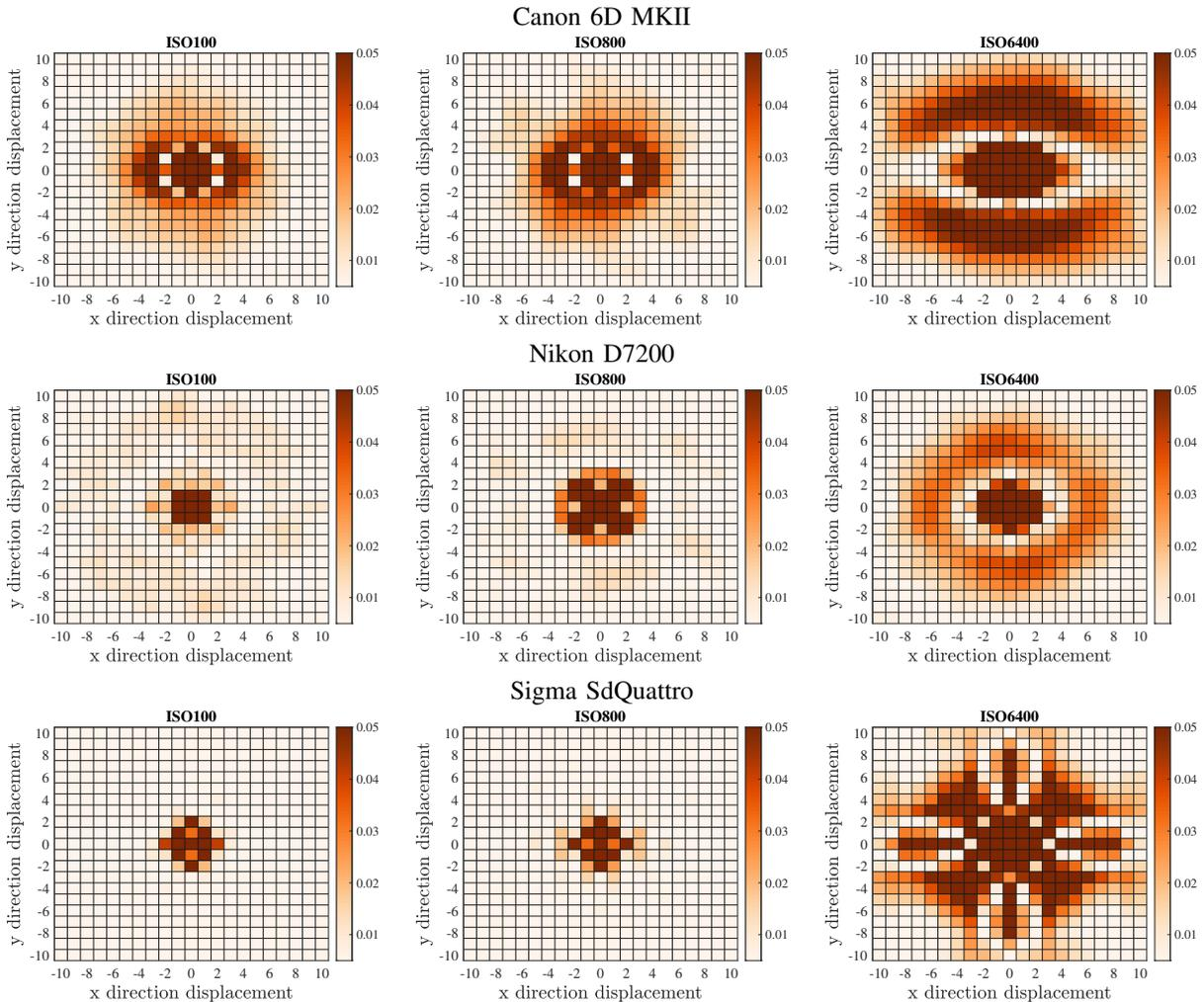
Fig. 2. The auto-correlation of noise residuals from images of different ISO speeds from 3 cameras. Rather than a single peak at  $(0,0)$ , auto-correlations have values spread over multiple pixel ranges. As the figure focuses on how far the spreading of auto-correlation reaches, the color bar focus on the range of  $[0, 0.05]$ . Values bigger than the upper limit 0.05 are also colored in dark brown.
