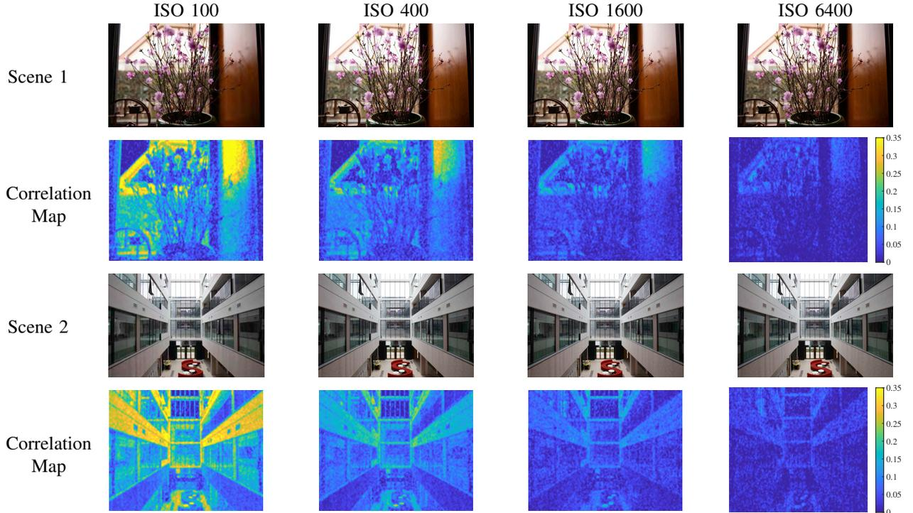
Fig. 4: Image of two different scene from a Canon 6D MKII from the Warwick Image Forensics Dataset. The images are taken with different ISO speeds. The exposure time for each image is set accordingly to let the images of the same scene have similar exposure level. The block-wise correlation maps are computed with a block size of  $128 \times 128$  pixels. The color bars used for the correlation maps are at the right hand side, next to the ISO 6400 correlation maps.
