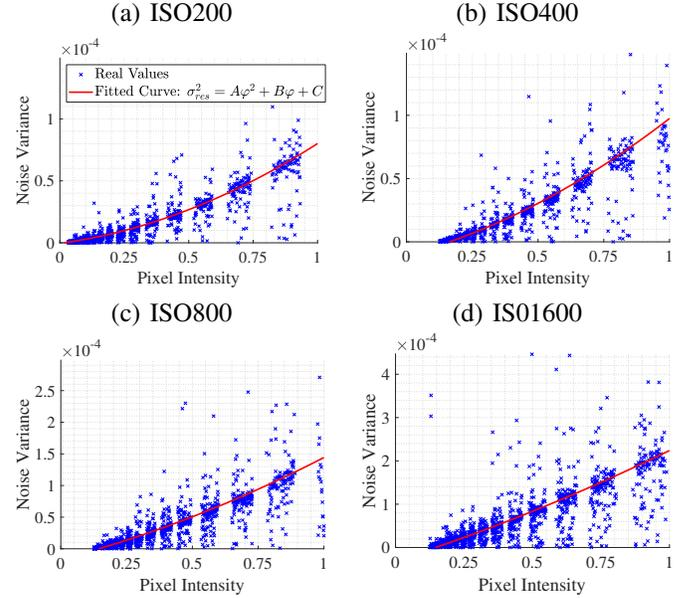
Fig. 2: Plots of noise’s variance  $\sigma_{res}^2$  against pixel intensity  $\varphi$  of images with different ISO speed from a Canon 6D MKII. We fit Equation (10) to the plots with a fixed second order coefficient,  $A = \sigma_k^2 = 5.24 \times 10^{-5}$ , estimated from Fig.1(b). The first order coefficient  $B$ , for the four fittings are: (a)  $B = 2.81 \times 10^{-5}$ , (b)  $B = 5.56 \times 10^{-5}$ , (c)  $B = 1.09 \times 10^{-4}$  and (d)  $B = 2.02 \times 10^{-4}$
