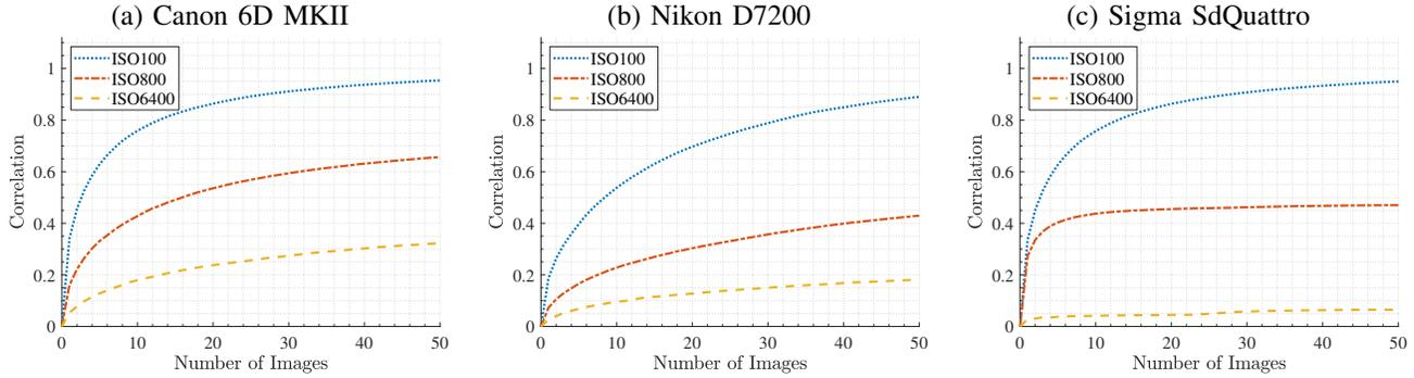
Fig. 1. The plots show how the number of JPEG images used for reference PRNU extraction may affect the quality of the extracted reference PRNU from three cameras: (a) Canon 6D MKII, (b) Nikon D7200 and (c) Sigma SdQuattro. We use the correlation between the extracted reference PRNU with another reference PRNU extracted from 100 flat-field images of ISO speed 100 to indicate the quality of the extracted reference PRNU.
