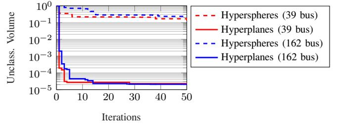
Fig. 2. For *case39\_epri* and *case162\_ieee\_dtc*, we compare the remaining unclassified volume between an infeasibility certificate based on hyperspheres from [8] and the proposed certificate in Section III-A2 based on hyperplanes. Note that these results cannot be directly compared to those of Table I, as here only the active generator set-points are assumed as degrees of freedom. In Table I, generator voltage set-points and uncertain injections are also considered.
