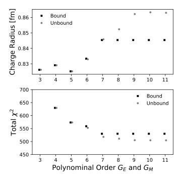
FIG. 4. Total  $\chi^2$  vs. the number of fit parameters in  $G_E$  and  $G_M$  using Eq. 4 and 5 for both the unbound and bound polynomial regressions of the 658 points of the rebinned Mainz dataset [13]. For these fits, by AIC and BIC,  $7^{th}$  order is the most appropriate for the bound regression while for the unbound  $9^{th}$  order is the most appropriate.
