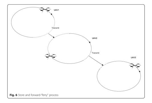
forward process is a reactive process—data are stored in the nodes and wait for the next hop to show up without knowing whether next hop will show up. T-OLSR takes all link exist and will establish into account in the route-finding process, and actively send the data to the nodes with knowing when target node will show up.
