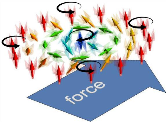
**Figure 10.** When a force is applied to a skyrmion, internal degrees of freedom are excited. These internal excitations lead to retardation effects which can be described as an effective mass of the skyrmion. Different forces lead to different types of deformations and therefore to different values of the effective mass. The figure is taken from Ref. [88].
