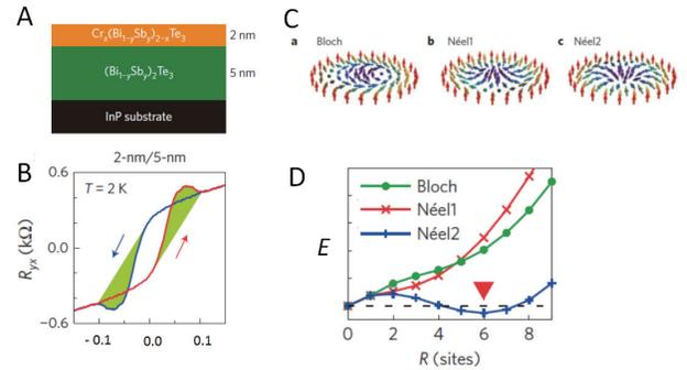
**Figure 20.** (A) The schematic structure of InP/TI/magnetic TI. (B) The experimental observation of the Hall resistance as a function of the magnetic field. The green shaded part corresponds to the topological Hall effect due to the skyrmion formation. (C) Three types of skyrmion. (D) Theoretical calculation results of the energy for each type of skyrmion. Reproduced from Ref. [188] with modification.
