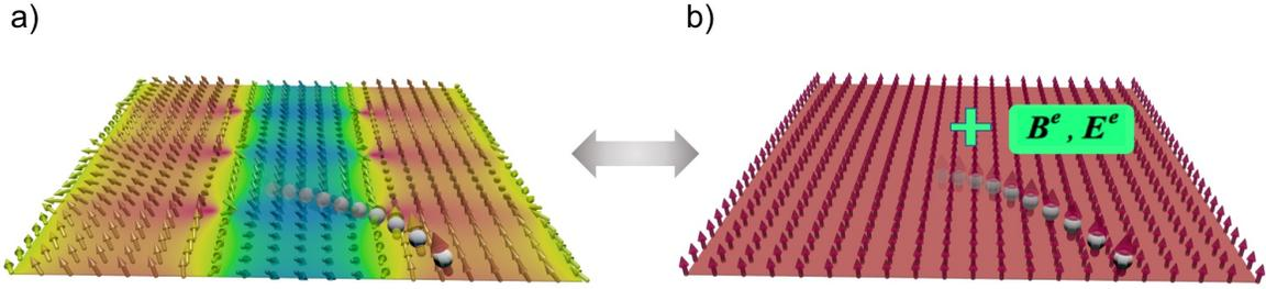
**Figure 8.** An electron traverses adiabatically a spatially inhomogeneous smooth magnetic texture. This problem can be mapped to one where the electron moves in a ferromagnetic background but instead “feels” additional emergent magnetic and electric fields.
