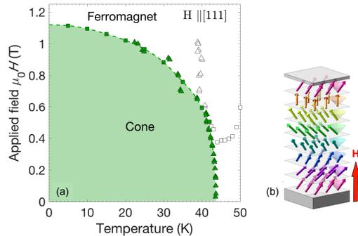
**Figure 13.** (a) Magnetic phase diagram of a 25.4 nm =  $1.83L_D$  thick MnSi(111) film grown on Si(111) derived from magnetometry measurements. The magnetic field  $H$  is applied along the film normal. An illustration of the cone phase is shown in (b). Adapted from Ref. [135].
