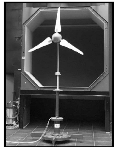
Fig. 6. (Right) Micro wind turbine placed in front of the nozzle of Open Jet Facility in TU Delft (left) plan drawing of the distances.
