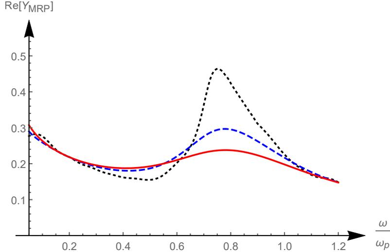
FIG. 2: Normalized real part of the admittance of the MRP for  $\kappa_{\max} = 20$ ,  $\lambda_{\max} = 15$ ,  $k_{\max} = 500$  and different collision frequencies  $\nu_0 \omega_p^{-1}$ : 0.05 (dotted), 0.15 (dashed), and 0.25 (bold).
