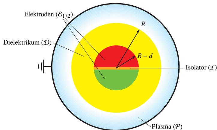
FIG. 1: Illustration of the idealized multiple resonance probe with powered electrodes  $\mathcal{E}_{1/2}$ , dielectric  $\mathcal{D}$ , and perturbed plasma  $\mathcal{P}$ . The radius of the electrodes is  $R - d$  and the thickness of the dielectric is  $d$ .
