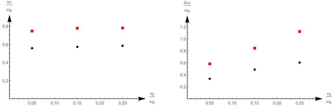
FIG. 3: Comparison of the resonance frequencies (left) and the half widths (right) of the **MRP** (squares) and the IP (dots) for three different collision frequencies  $\nu_0\omega_p^{-1}$ : 0.05, 0.15, and 0.25.
