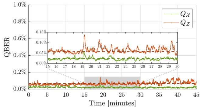
FIG. 2. **Intrinsic QBER and temporal stability of the POGNAC polarization encoder.** The average QBER measured for the key-generation basis was  $Q_{\mathcal{Z}} = 0.07 \pm 0.02\%$  (dashed red line) while an average  $Q_{\mathcal{X}} = 0.02 \pm 0.01\%$  (dashed green line) was measured for the control basis. A close-up between minutes 15 to 30 can be seen in the inset plot.
