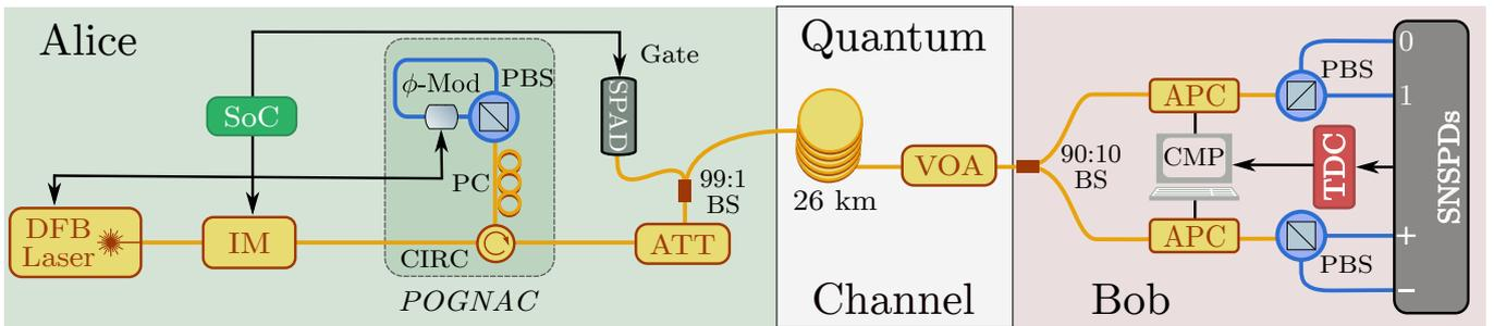
FIG. 1. **Experimental Setup.** For a detailed description see Sec. II. Single Mode fibers are indicated in yellow while Polarization Maintaining fibers in blue.
