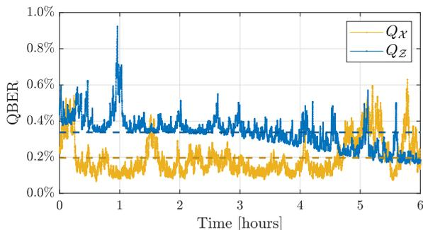
FIG. 3. **QBER measurement for a 6 hour long acquisition along a 26 km optical fiber channel.** The average QBER measured for the key-generation basis was  $Q_Z = 0.3 \pm 0.1\%$  (dashed blue line) while an average  $Q_X = 0.2 \pm 0.1\%$  (dashed yellow line) was measured for the control basis.
