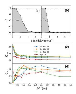
Figure 2: (a-b) Correlation coefficient squared for increasing delay (forgetting curves) for the STM and PC tasks. Data here are for  $\theta^{int}$  equal to 0.3 and 1  $\mu$ s respectively. (c) The STM capacity versus  $\theta^{int}$  for different gain levels. The data 'w/o YIG' corresponds to the STM capacity of the electronic components alone. (d) Same as (c) but for the PC task
