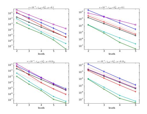
Figure 3: LPS with global grad-div stabilization,  $P_3/P_3$  pair of finite element spaces, Grid 1 (left) and Grid 2 (right), dotted line: slope for third order convergence, same legend as in Figure 2.
