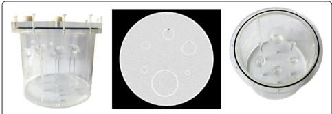
**Fig. 1** The phantom used to determine the recovery coefficients. The second image is a CT slice of the phantom on which the order of the spheres can be seen
