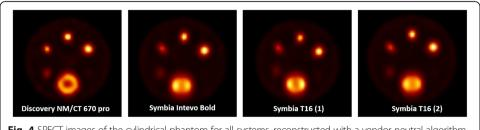
Fig. 4 SPECT images of the cylindrical phantom for all systems, reconstructed with a vendor-neutral algorithm
