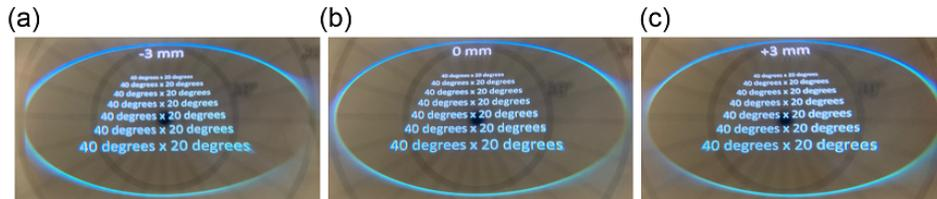
Fig. 12. Eye box measurement results: The  $40^\circ \times 20^\circ$  image captured at (a) the left-most, (b) the center, (c) the right-most position. Note that the FOV panel was captured together to show the FOV. The measured eye box was  $6 \times 4 \text{ mm}^2$ .
