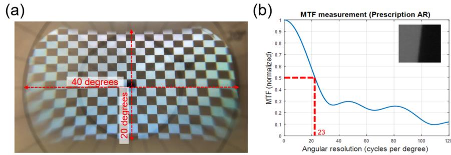
Fig. 11. Experimental results of the FOV and resolution measurement: (a) The AR image covers  $20^\circ$  by  $40^\circ$  of the checking board in vertical and horizontal direction respectively. (b) The analysis of slant-edge measurement at center field. Note that the angular resolution of 23 CPD is realized in our prototype.
