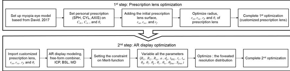
Fig. 2. Flow chart of the two-step optimization for Prescription AR: The frontal and rear surfaces ( $S_f, S_r$ ) are optimized at given lens thickness  $t_l$  in the first step based on user's prescription. Other geometric parameters ( $R_{l1}, R_{l2}, R_{cy}, a, d_p, t_{BSL}, t_c, t_w, \theta_d, \theta_l, \theta_p, \theta_c, \theta_w$ , and  $\theta_{free}$ ) are optimized in the second step based on target foveated resolution and eye relief range,  $d_e$ .
