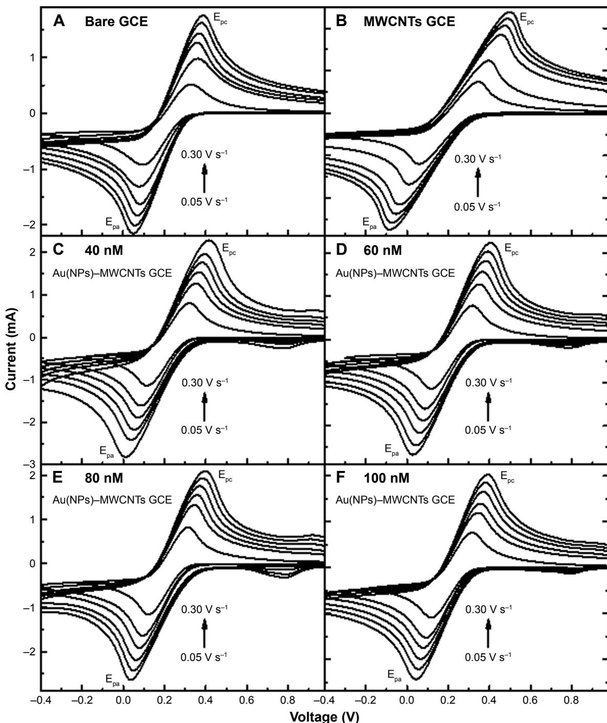
**Figure 2** CV scans of GCE, MWCNTs-modified GCE, and Au(NP)-MWCNT-modified GCE in  $0.1 \text{ mol L}^{-1} \text{ K}_3[\text{Fe}(\text{CN})_6]$  with scan rates 0.05, 0.1, 0.15, 0.2, 0.25, and  $0.3 \text{ V s}^{-1}$ . **Note:** (A) GCE, (B) MWCNT-modified GCE, (C) 40 nM Au(NP)-MWCNT-modified GCE, (D) 60 nM Au(NP)-MWCNT-modified GCE, (E) 80 nM Au(NP)-MWCNT-modified GCE, and (F) 100 nM Au(NP)-MWCNT-modified GCE.
