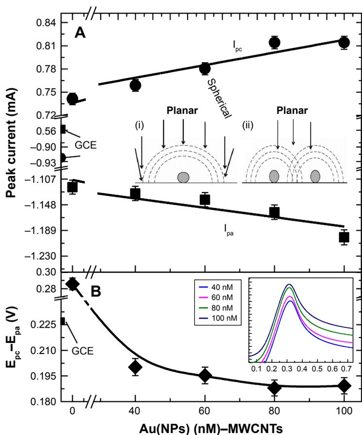
**Figure 5** Plots of redox currents ( $I_{pa}$ ,  $I_{pc}$ ) and  $\Delta E (=E_{pc} - E_{pa})$  as a function of Au(NPs) concentrations in Au(NP)–MWCNT nano hybrids for complete understanding about symmetry of CV profile due to formation of diffusion zone around Au (NPs).
