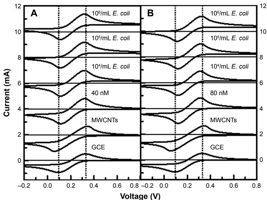
**Figure 7** CV plots of the Au(NP)-MWCNT-modified GCE in  $0.1 \text{ mol L}^{-1} \text{ K}_3[\text{Fe}(\text{CN})_6]$  at  $0.05 \text{ V s}^{-1}$  for different concentrations of *Escherichia coli*  $10^4$ ,  $10^5$ , and  $10^6/\text{mL}$ . **Note:** (A) 40 nM Au(NP)-MWCNT-modified GCE, and (B) 80 nM Au(NP)-MWCNT-modified GCE.
