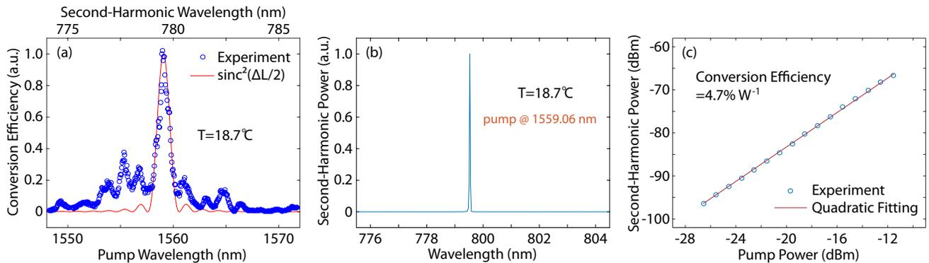
FIG. 3. SHG from a straight LN nanophotonic waveguide with a length of 8 mm. (a) Conversion efficiency spectrum at  $T=18.7^\circ\text{C}$ , with the center wavelength of the  $\text{sinc}^2$ -function aligned to the measured peak. (b) SHG spectrum at a fixed pump wavelength of 1559.06 nm at  $T=18.7^\circ\text{C}$ . (c) Second-harmonic power as a function of pump power, with experimental data compared with a quadratic fitting, exhibiting a conversion efficiency of  $4.7\% \text{ W}^{-1}$ .
