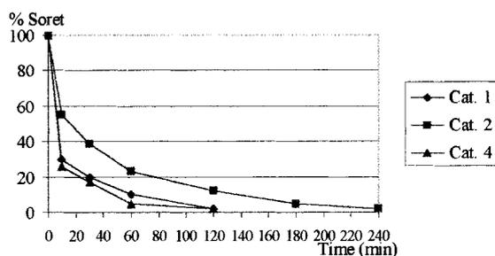
**Fig. 2.** Time variation of the Soret band of the catalysts **1**, **2** and **4**.
