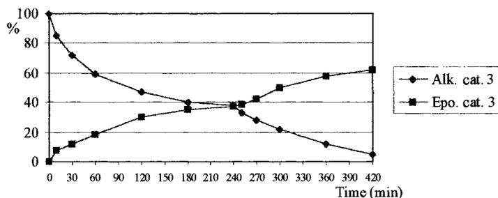
**Fig. 3.** Substrate and product evolution in the epoxidation of 1-methyl-cyclohexene with catalysts **3**. (1 mmol of metalloporphyrin, 100 mmol of 1-methyl-cyclohexene, 20 mmol of pyridine and 2 mmol of tetrabutylammonium bromide, 20 ml of NaOCl 0.6 M.).
