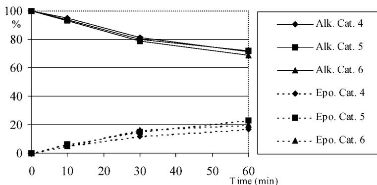
Fig. 5. Substrate and product evolution in the epoxidation of 1-methyl-cyclohexene with catalysts 4, 5 and 6, until full catalyst degradation. (1 mmol of metalloporphyrin, 100 mmol of 1-methyl-cyclohexene, 20 mmol of pyridine and 2 mmol of tetrabutylammonium bromide, 10 ml of NaOCl 0.6 M.).
