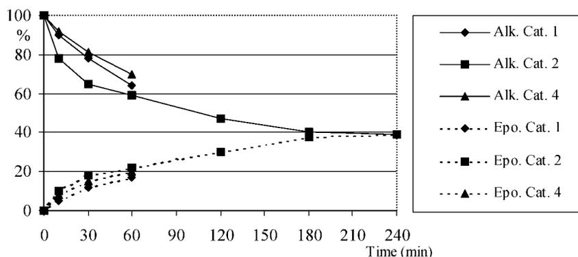
**Fig. 1.** Substrate and product evolution in the epoxidation of 1-methyl-cyclohexene with catalysts **1**, **2** and **4**, until total catalyst degradation. (1 mmol of metalloporphyrin, 100 mmol of 1-methyl-cyclohexene, 20 mmol of pyridine and 2 mmol of tetrabutylammonium bromide, 10 ml of NaOCl 0.6 M.).
