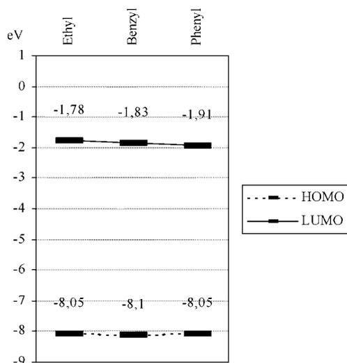
Fig. 8. HOMO and LUMO values (eV) for the porphyrins 4, 5 and 6. Values from Hyperchem v.3 using the semi-empirical AM1 with a Polak–Ribiere algorithm. Final gradient of 0.01 Kcal  $\text{\AA}^{-1} \text{mol}^{-1}$ .
